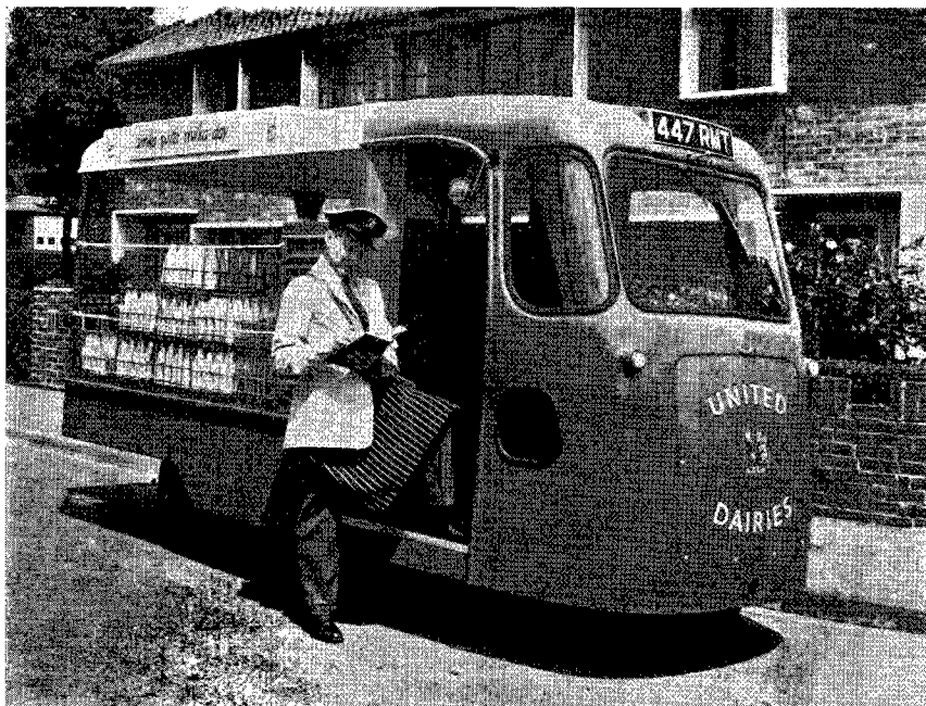
FIG. 4 LATEST-STYLE ELECTRIC DELIVERY VEHICLE WITH FIBRE-GLASS BODY-WORK
